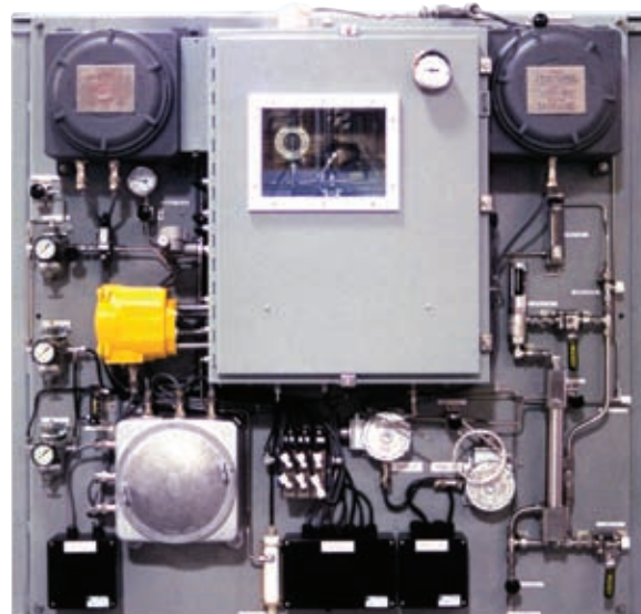
Model 4650 H 2 S in Lean Amine Analyzer
